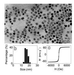
Figure 1. (a) TEM image of the PEG-coated  $Fe_3O_4$  nanoparticles, (b) size distribution of the particles shown in frame a, (c) room-temperature magnetization curve of the PEG-coated  $Fe_3O_4$  nanoparticles.
