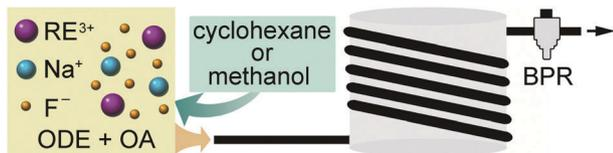
Scheme 1 Sketch of the flow synthesis of NaGdF<sub>4</sub>:Yb,Er nanocrystals.
