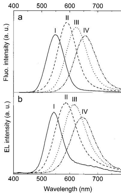
FIG. 4. (a) Fluorescence spectra of CdTe aqueous solutions excited at 400 nm. (b) Electroluminescence spectra of (CdTe/PDDA)\*30 films. The spectra recorded from CdTe I, CdTe II, CdTe III and CdTe IV were labeled I, II, III, and IV, respectively.
