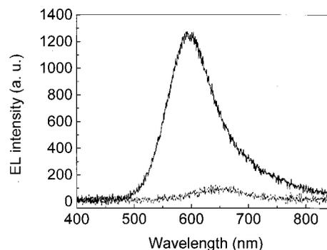
FIG. 6. Electroluminescence spectra of two-layer films consisting of two different sized nanocrystals: spectrum in solid line was recorded from ITO//PEI(CdTe II/PDDA)\*20/(CdTe IV/PDDA)\*20//Al, spectrum in dashed line from ITO//PEI(CdTe IV/PDDA)\*20/(CdTe II/PDDA)\*20//Al. The EL emissions were recorded under the same current densities with positive terminal of power source connected to the ITO electrode.
