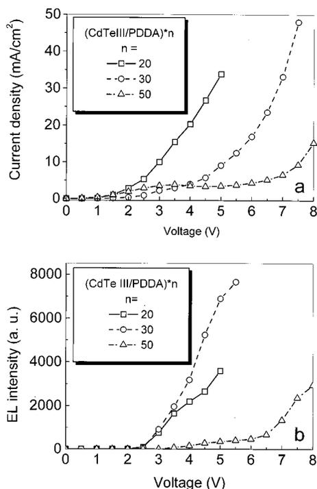
FIG. 2. (a)  $I$ - $V$  characteristics of  $(\text{CdTe III/PDDA})^*n$  films sandwiched between ITO and aluminum electrodes, with  $n=20, 30, 50$ . (b) Electroluminescence intensities of the above films vs externally applied voltage.
