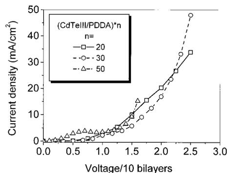
FIG. 3. Current densities of the films of  $(\text{CdTe III/PDDA})^*n$  with  $n=20, 30$ , and 50 vs electric field. The electric field was expressed in units of voltage/ten bilayers.
