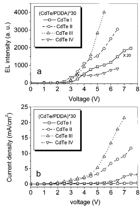
FIG. 5. (a) The electroluminescence intensities vs applied voltages from 30-bilayer CdTe/PDDA films consisting of different size nanocrystals, namely, CdTe I, CdTe II, CdTe III, and CdTe IV. (b) The corresponding  $I$ - $V$  characteristics.
