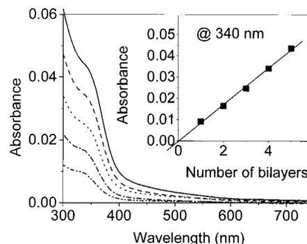
FIG. 1. Absorption spectra of one-, two-, ..., five-bilayer of CdTe/PDDA films. The pH value of the CdTe solution was controlled at 6.3 ± 0.2 during the film preparation. (Insert) Absorbance at the shoulder position of 340 nm vs the number of bilayers.
