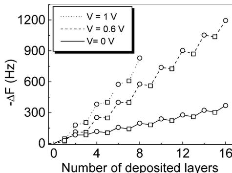
**Fig. 2** Frequency decrease ( $-\Delta F$ ) induced by the EFDLA deposition of (PDDA/CdTe) $_n$  films on the QCM electrode at different working voltages, *i.e.*, 0 V, 0.6 V and 1.0 V. The deposition under 0 V corresponds to the traditional LbL self-assembling process. Squares and circles represent frequency changes recorded after the deposition of PDDA and CdTe, respectively.
