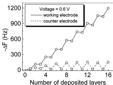
**Fig. 1** Frequency decrease ( $-\Delta F$ ) caused by deposition of (PDDA/CdTe) $_n$  films on the QCM electrode by the EFDLA method. The working voltage is 0.6 V. Squares and circles represent frequency changes recorded after depositions of PDDA and CdTe, respectively.
