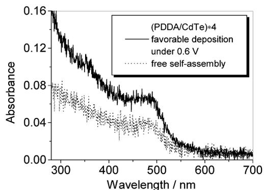
**Fig. 3** Reflective UV-Visible spectra of (PDDA/CdTe)\*4 films deposited on gold surfaces by (a) the LbL self-assembly method, (b) favorable EFDLA deposition with a working voltage of 0.6 V.
