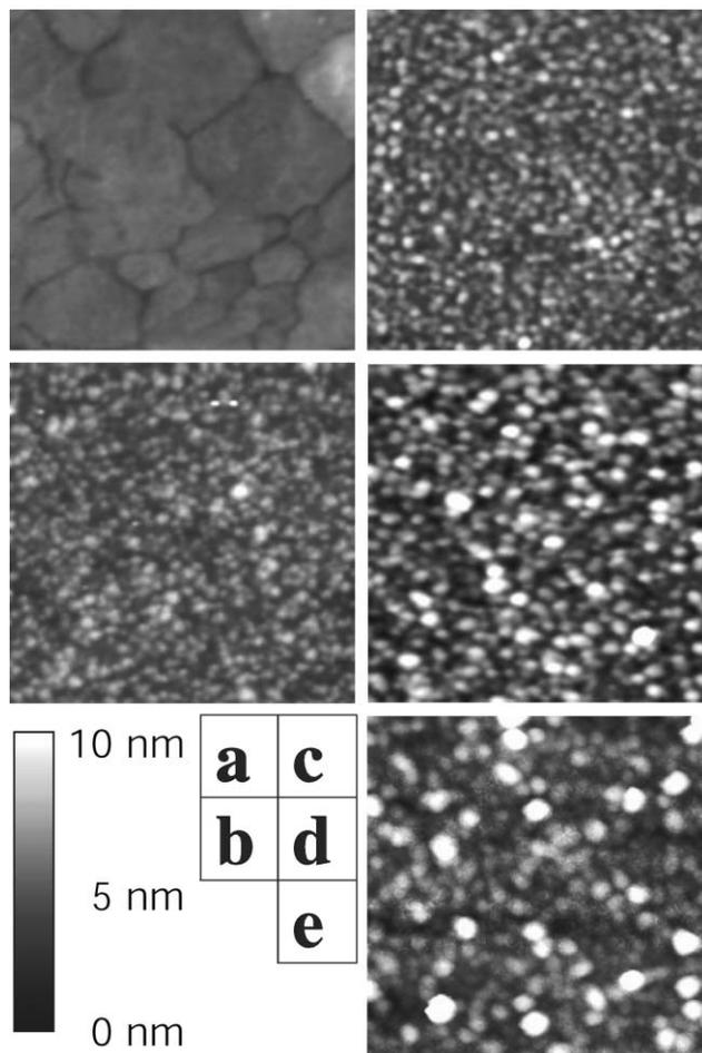
**Fig. 4** AFM images: a, bare Au electrode; b, (PDDA/CdTe)\*6 film on the counter electrode,  $V = 0.6 \text{ V}$ ; c, d, and e, (PDDA/CdTe)\*6 films on the working electrode,  $V = 0, 0.6 \text{ V}$  and  $1.0 \text{ V}$ .
