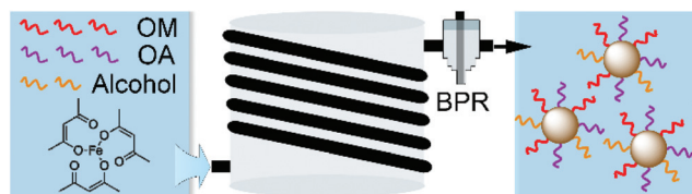
Scheme 1 Sketch of the flow synthesis of \text{Fe}_3\text{O}_4 nanocrystals. BPR represents a back pressure regulator.
