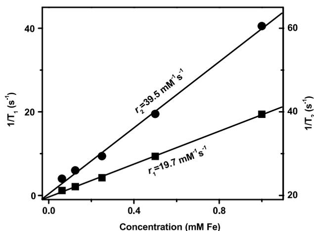
**Figure 6.**  $T_1$  and  $T_2$  relaxation rates ( $1/T_{1,2}$ ) plotted against the Fe concentrations of the 5.4 nm SPIONs (1.5 T, 37 °C).
