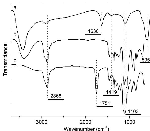
**Figure 4.** FTIR spectra of (a) the 5.4 nm SPIONs, (b) TREG and (c) HOOC-PEG-COOH.
