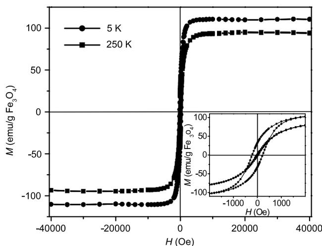
**Figure 5.** Magnetization ( $M$ ) loops for the 5.4 nm SPIONs measured at 5 and 250 K. The inset shows an expanded view of the low magnetic field behavior for both temperatures.
