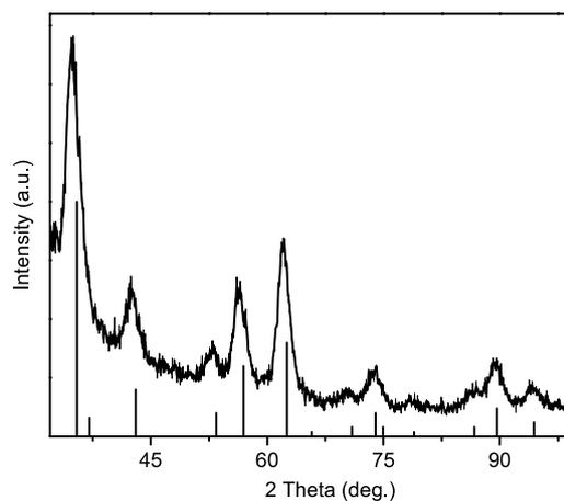
**Figure 2.** Powder x-ray diffractogram of the 5.4 nm SPIONs. Bottom: JCPDS card (19-0629) data for magnetite.
