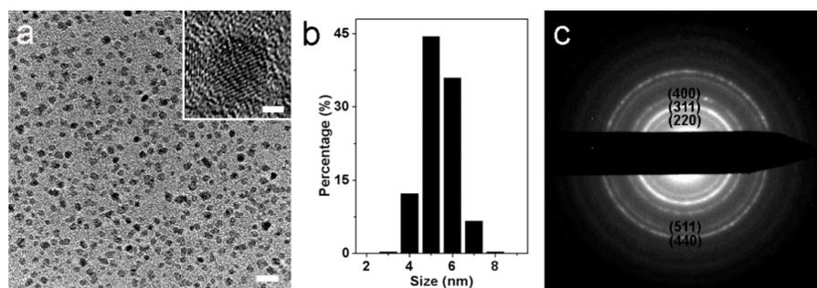
**Figure 1.** (a) TEM (inset is HR-TEM) images, (b) size distribution histogram and (c) electron diffraction patterns of the 5.4 nm SPIONs. The scale bar is 20 nm in the TEM image and 2 nm in the HR-TEM image.
